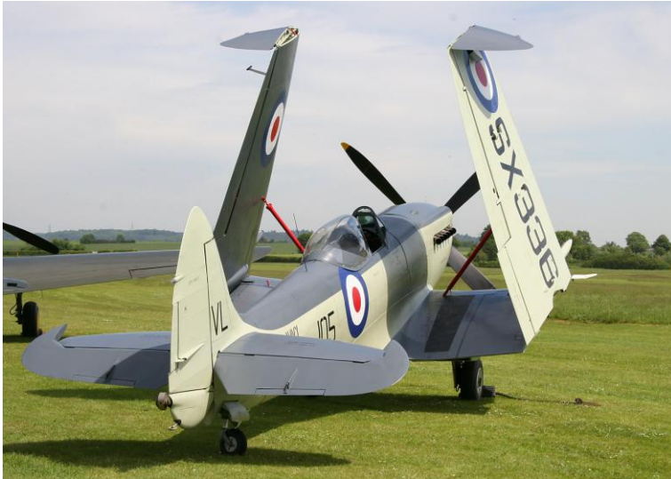
Supermarine Spitfire XVII SX336 at Old Warden 4 June 2006 with wings folded, showing bubble canopy and arrestor hook under rudder [Photo –Peter Arnold Collection]
