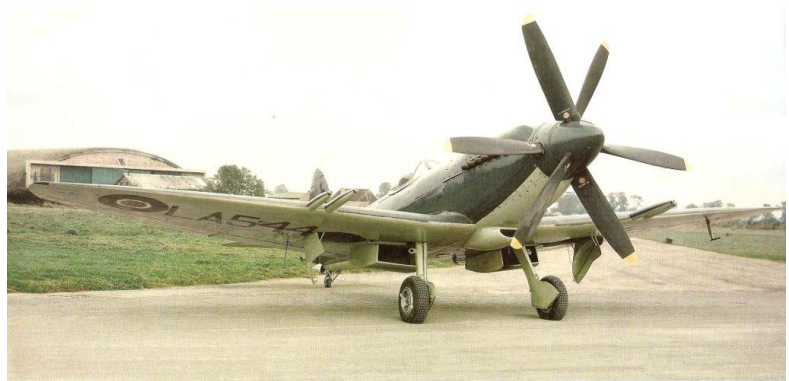
Supermarine Seafire 46 with contra-rotating propeller. This was the actual aircraft I flew – LA544
