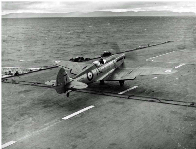
Seafire XV on takeoff has just passed over one of the lowered safety barriers. Flaps can be seen at the 18 degree position—aileron are slightly left wing down to counteract propeller torque. Rudder trim tab is set right, rudder slightly left also to counteract torque. ‘T’ on tail designates carrier HMS Theseus
